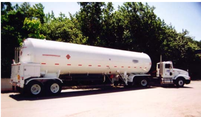
MC-338 Cargo Tank (vacuum jacketed)
