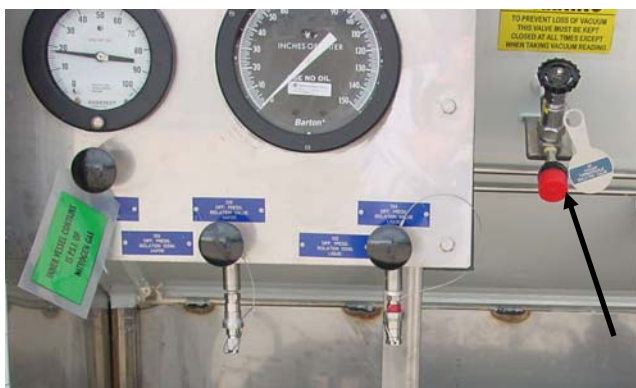
Thermocouple tube connection and isolation valve for tank car
